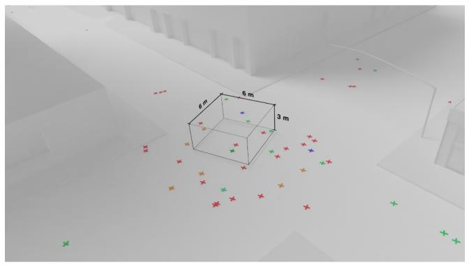
Fig 9: A measurement volumes (Sample point A) used to determine airborne concentrations
