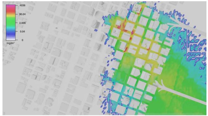
Fig 11: The simulated ground deposition of CS particles, following the prevailing wind
