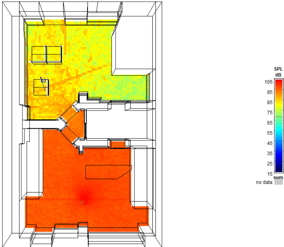
Figure 5.5: Sound pressure level spread in the Kassel Internet Café model computer simulation (A-weighted).
